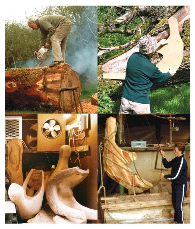
Unforeseen problems included the timber having a moisture content of 60% – for timber not to crack, its moisture content has to be no more than 10%, and the resulting process of doing that is both slow and tedious. Michael initially brought samples of wood to three commercial kilns, which proved unsuccessful. He was left with only one option – to build his own kiln.
